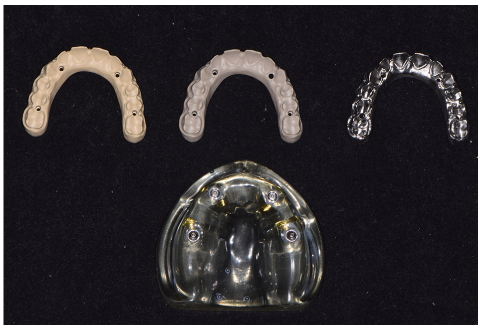
Fig. 1. Typodont model and frameworks: Evaluated frameworks milled from PEEK, PEKK and titanium (left to right), and the typodont model.
