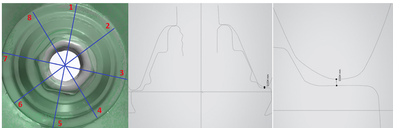
Fig. 3. Evaluation of marginal fit: Four cross-sections and eight points (left) to evaluate the marginal fit. The closest distance was between the implant and abutment was visually determined (middle) on the enlarged cross-section (right).
