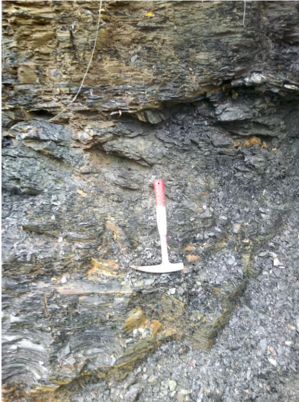
Figure C-26 – SWC-111,112,113 – Internal decollement in the Marcellus, Newton-Hamilton quarry, PA. Photo by author at 40.398°N, 77.826°W.
