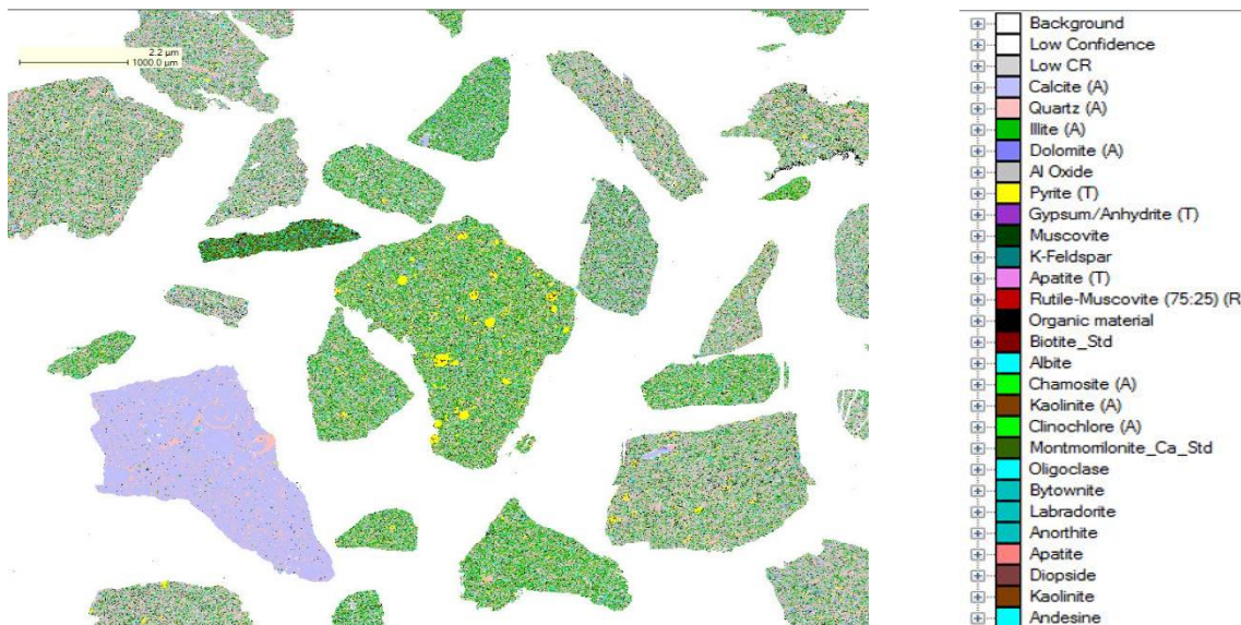
Figure 3-30 – QEMScan false color image of section from core of pilot well Hamilton 1 ( sample SWC-139)
