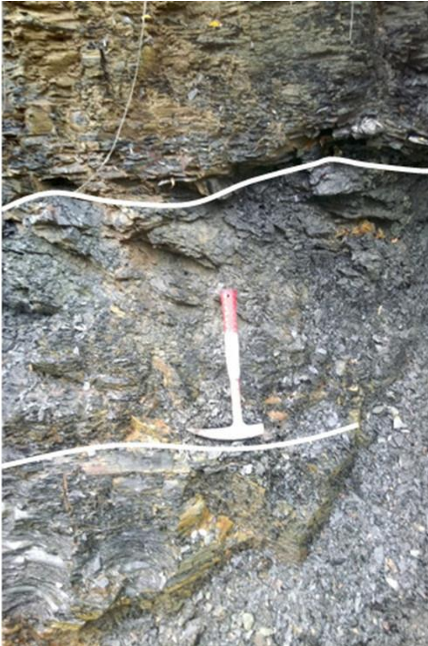
Figure 3-20 -- Shear zone within the lower Marcellus formation at the Newton-Hamilton quarry.
