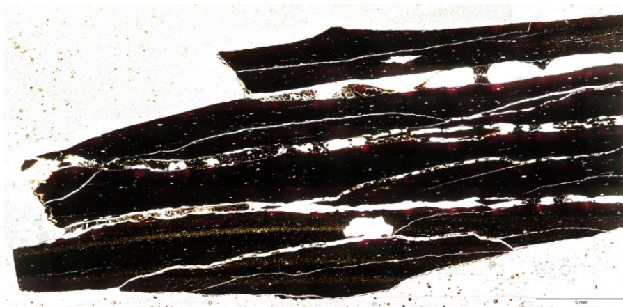
Figure 3-6 -- Marcellus organic-rich shale; sample SWC-056 from a quarry near Elimsport, PA. The scale at the bottom right is 5mm
