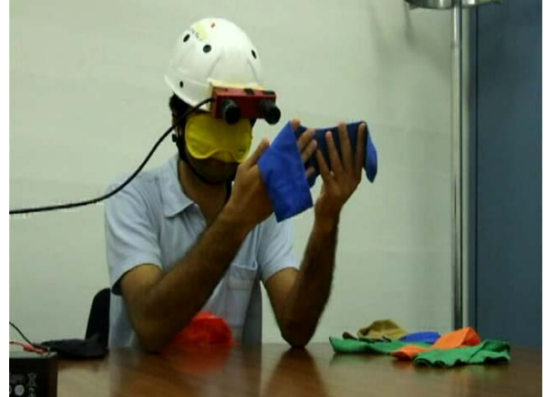
Fig. 5. A blindfolded participant scrutinizing a blue sock with a stereoscopic camera mounted on his head.
