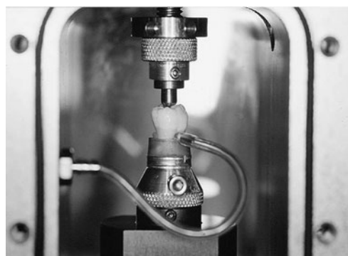
Fig. 1 Fatigue apparatus used to simulate cyclic masticatory stresses and pulpal pressure. Samples are mounted on a semi-rigid rubber base to allow for sliding movements such as encountered in natural dentition. Detailed view of one of the eight chambers of the fatigue device
