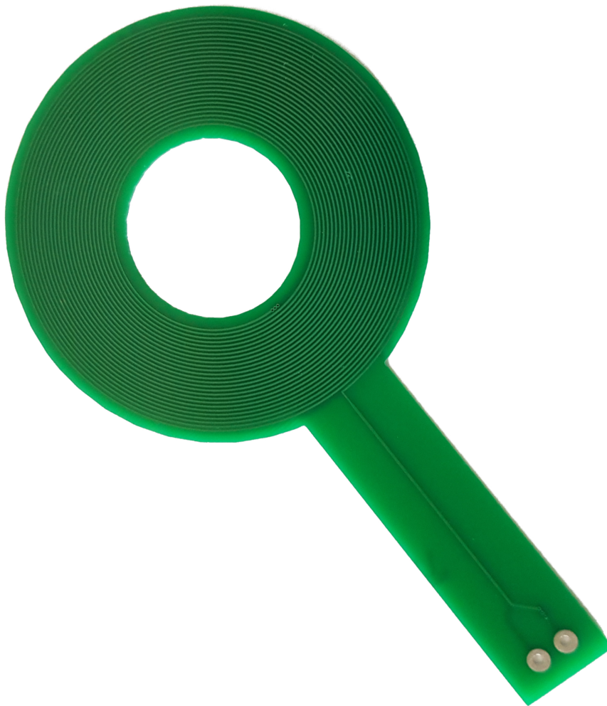
Figure 2.1 Detailed picture of a double layered printed circuit board shim coil.
