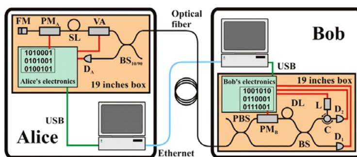
**Figure 2.** Schematic of the p&p prototype.
