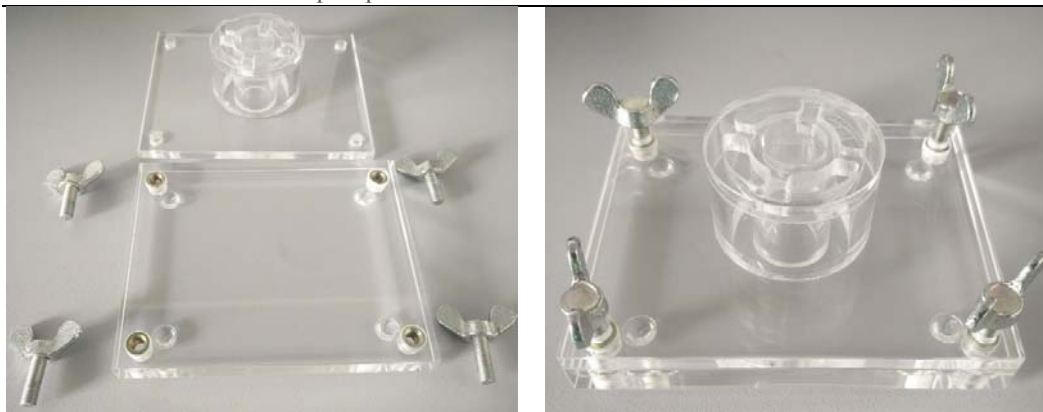
Figure S5. Photographs of a) individual components of the concentric set-up b) working model of the set-up.
