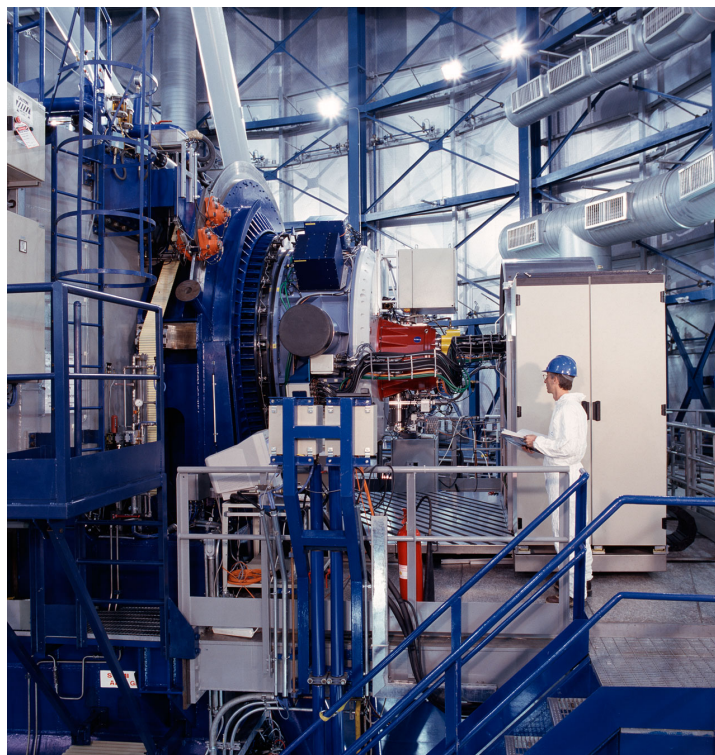
Fig. 6.1 NACO attached to the Nasmyth focal point on VLT's UT1. Image credit: ESO.
