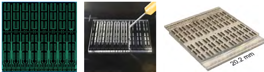
Figure 6.13: Capacitive test chip design (left), glue deposition (center) and final assembly (right).
