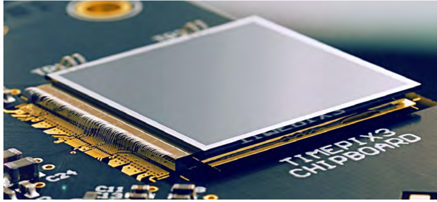
Figure 4.21: Picture of a silicon planar sensor bump-bonded to the Timepix3 ROC below, wire-bonded to the chip-carrier board [95].
