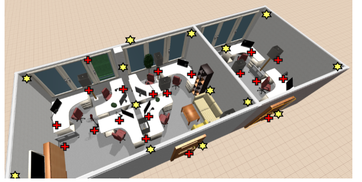
Fig. 3: Office Environment of implementation. The "cross" represents the electrical-electronic interface and the "star" the sensors for monitoring the environment.
