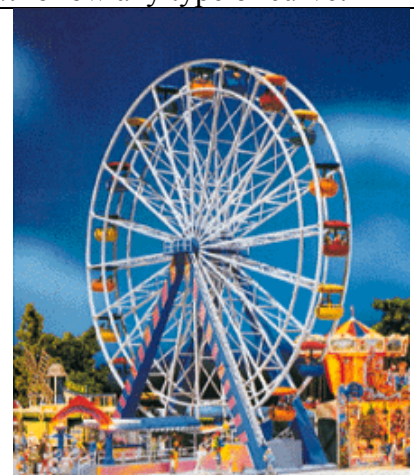
Figure 2. Ferris Wheel: the prototypical example of a circular movement of translation, often confused with a movement of rotation
