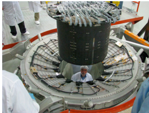
Figure 4.14: AMS-02 assembly trial: insertion of the Inner Tracker in the magnet vacuum case.
