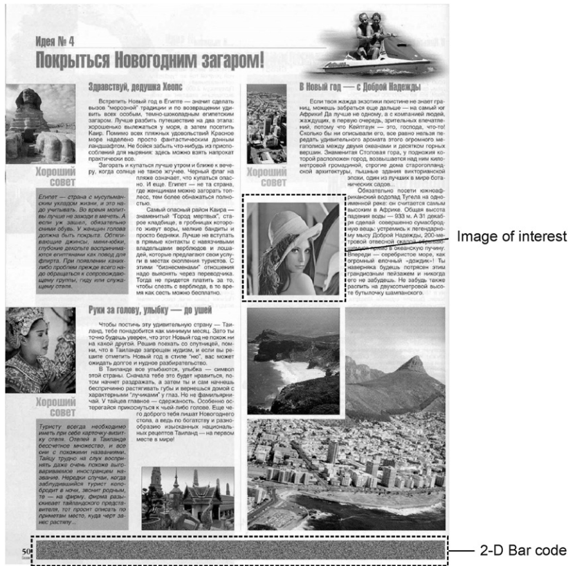
Fig. 1. Visual communications via printing channels: example of journal with side information communications in the form of 2-D bar code.
