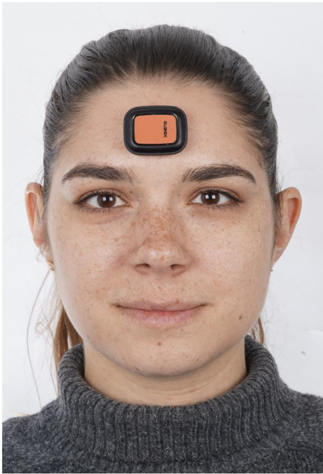
Figure 1. Head posture was recorded using a triaxial IMU - inertial measurement unit (SENS motion®, SENS Innovation ApS, Denmark) capable of capturing real-time three-dimensional orientation data (pitch, roll, and yaw angles). The IMU was calibrated on a horizontal surface prior to each recording to define a neutral position (0° for each axis). The sensor was affixed to the participant's forehead using a hypoallergenic double-sided adhesive tape, ensuring it was positioned parallel to the bipupillary line. This placement allows accurate registration of head orientation while minimizing measurement errors associated with sensor misalignment, as previously validated in earlier methodological studies (Al-Yassary et al., Sci Rep 2021 [18]; Al-Yassary et al., J Oral Rehabil 2022 [17]). Participants were seated in a standardized 90–90–90 posture (hips, knees, and ankles flexed at 90°) and instructed to look at their own eyes in a mirror for 30 seconds to establish a mirror-guided natural head posture. The mirror was then covered, and participants maintained their self-balanced head posture for 5 minutes without visual feedback. Throughout this period, the IMU continuously recorded angular displacements of the head in three axes: pitch (anteroposterior inclination; flexion/extension), roll (lateral tilting; right/left inclination), and yaw (horizontal rotation; right/left turning). The collected data were subsequently averaged over the 5-minute recording period to provide a stable representation of each participant's natural head posture.
