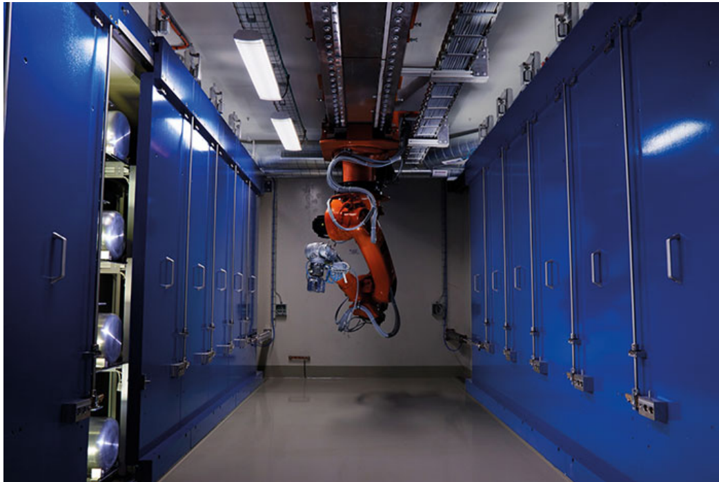
Figure 3. Robot for remote handling (in the center) and the storage shelves for ISOLDE and CERN-MEDICIS targets. Photo courtesy of : [36].
