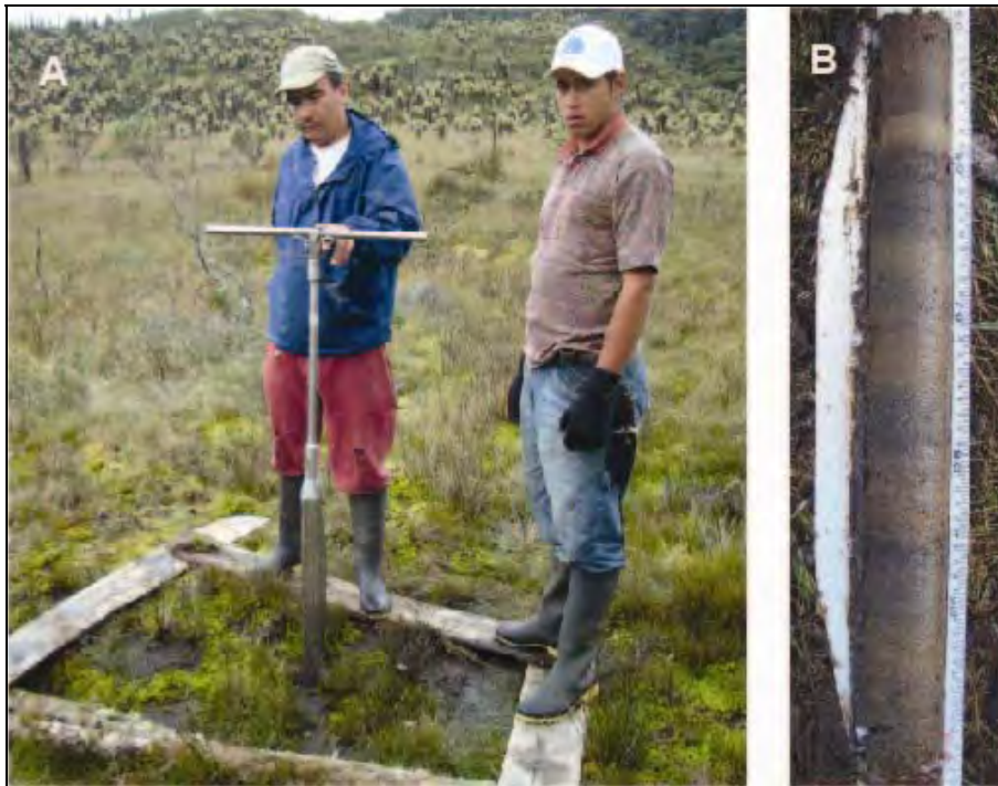
Fig. 3.3. A) Russian corer ready for use; B) example of a 50 cm long half core.
