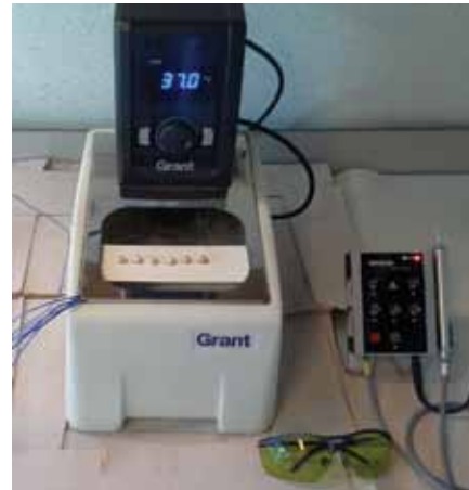
FIG. 1 Tooth samples mounted on a platform and immersed in 37°C water bath.
