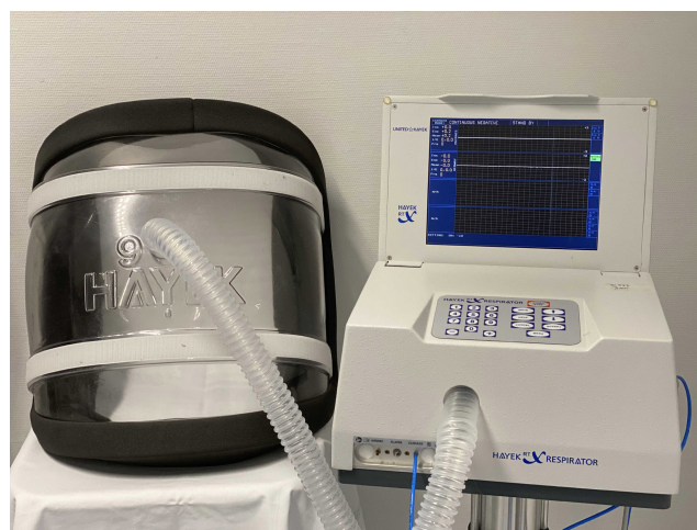
FIGURE 3 Hayek RTX Biphasic Cuirass Ventilator. The ventilator is connected to the cuirass shell with a tubing. The flexible cuirass shell is available in different sizes ranging from small neonatal size to large adult size [Colour figure can be viewed at wileyonlinelibrary.com ]
