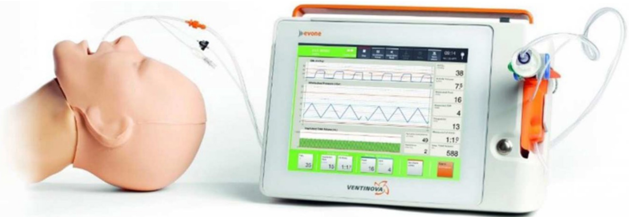
FIGURE 2 Evone ventilator (Ventinova Medical B.V., Eindhoven, the Netherlands) connected to a mannequin with the Tritube for flow-controlled ventilation. Reproduced with permission from 48 [Colour figure can be viewed at wileyonlinelibrary.com ]
