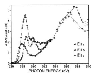
FIG. 5. O 1s absorption spectrum of YBa<sub>2</sub>Cu<sub>3</sub>O<sub>6.95</sub> for polarizations E||a, E||b, and E||c. Above 533 eV the cross sections are almost independent of x.
