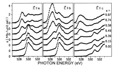
FIG. 3. O 1s absorption spectra of  $YBa_2Cu_3O_x$  for E||a, E||b, and E||c.
