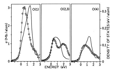
FIG. 9. Comparison of experimental atomic O 1s cross sections (symbols) with LDA-band-structure calculated DOS for YBa<sub>2</sub>Cu<sub>3</sub>O<sub>7</sub> as obtained by Zaanen *et al.* (Ref. 64).
