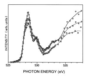
FIG. 2. Demonstration of corrections for the polarized O 1s absorption spectrum  $(\mathbf{E}\|b)$  for YBa<sub>2</sub>Cu<sub>3</sub>O<sub>6.95</sub>. Squares, noncorrected data; diamonds, data corrected for the intensity variation of the primary beam  $I_0$ ; and circles, fully corrected data including self-absorption corrections.
