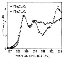
FIG. 7. Comparison of O 1s absorption spectra for  $\mathbf{E} \| a$  of  $YBa_2Cu_3O_7$  and  $YBa_2Cu_4O_8$ .
