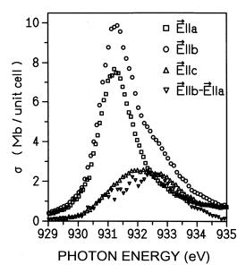
FIG. 12. Cu  $2p_{3/2}$  absorption spectrum of YBa<sub>2</sub>Cu<sub>3</sub>O<sub>6,97</sub> for polarizations  $\mathbf{E}||a$ ,  $\mathbf{E}||b$ , and  $\mathbf{E}||c$ . The difference of the cross sections for  $\mathbf{E}||b$  and  $\mathbf{E}||a$  is nearly equal to the  $\mathbf{E}||c$  spectrum.
