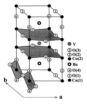
FIG. 1. Unit cell of YBa<sub>2</sub>Cu<sub>3</sub>O<sub>7</sub>. The CuO<sub>2</sub> planes and the CuO<sub>3</sub> chains are indicated by a grey tone.
